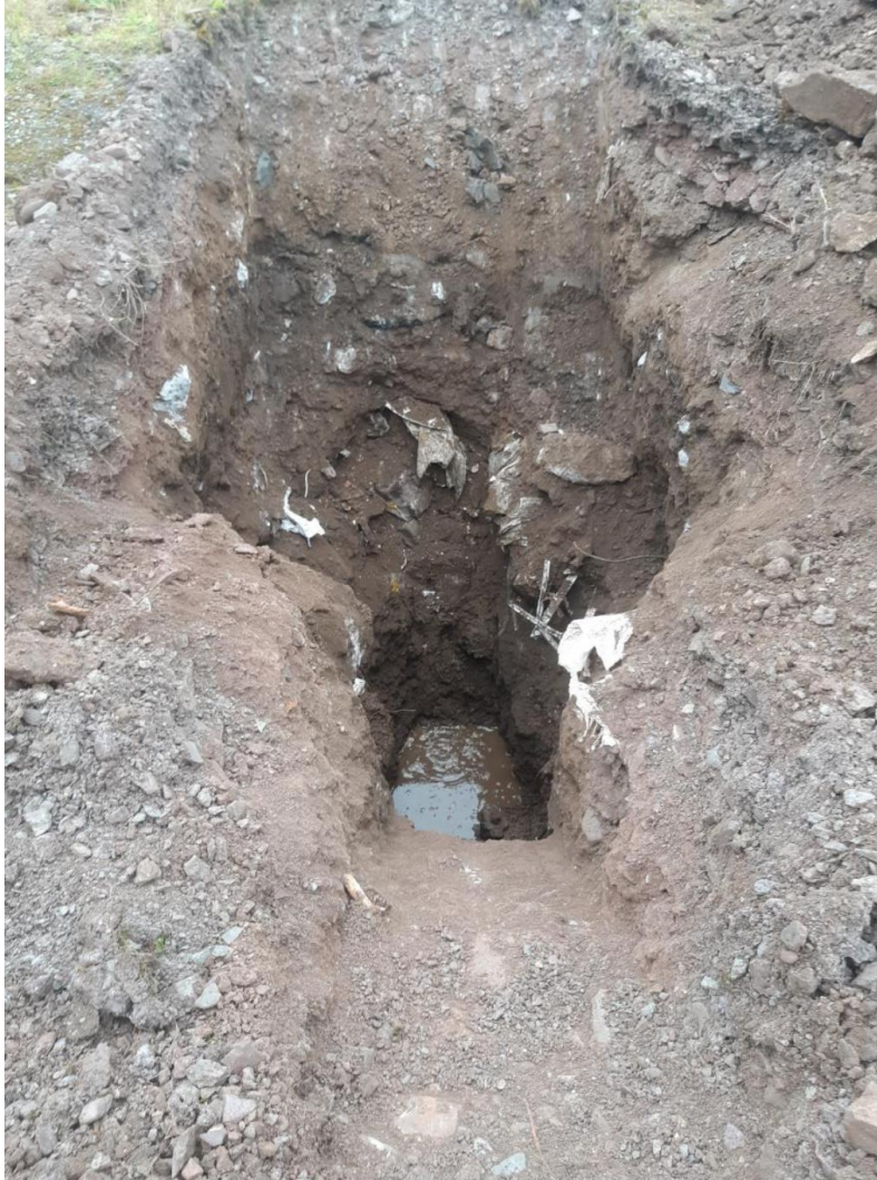
Figure 13.13 TP08 C&D waste
