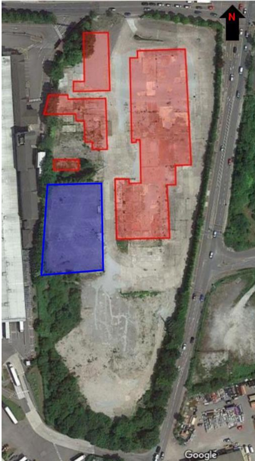
Figure 5.3: Extract from Google Maps marked up to show existing concrete ground slabs and foundations | red: concrete floor slabs/ foundations, blue: carpark | not to scale
