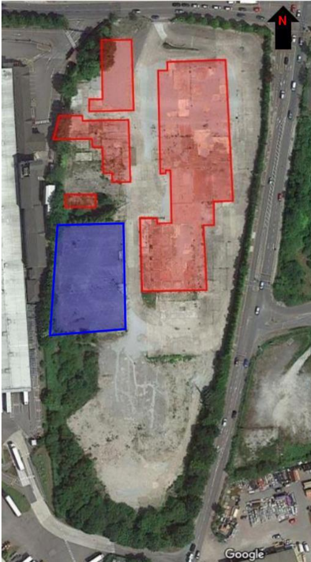
Figure 15.4: Extract from Google Maps marked up to show existing concrete ground slabs and foundations | red: concrete floor slabs/ foundations, blue: carpark | not to scale
