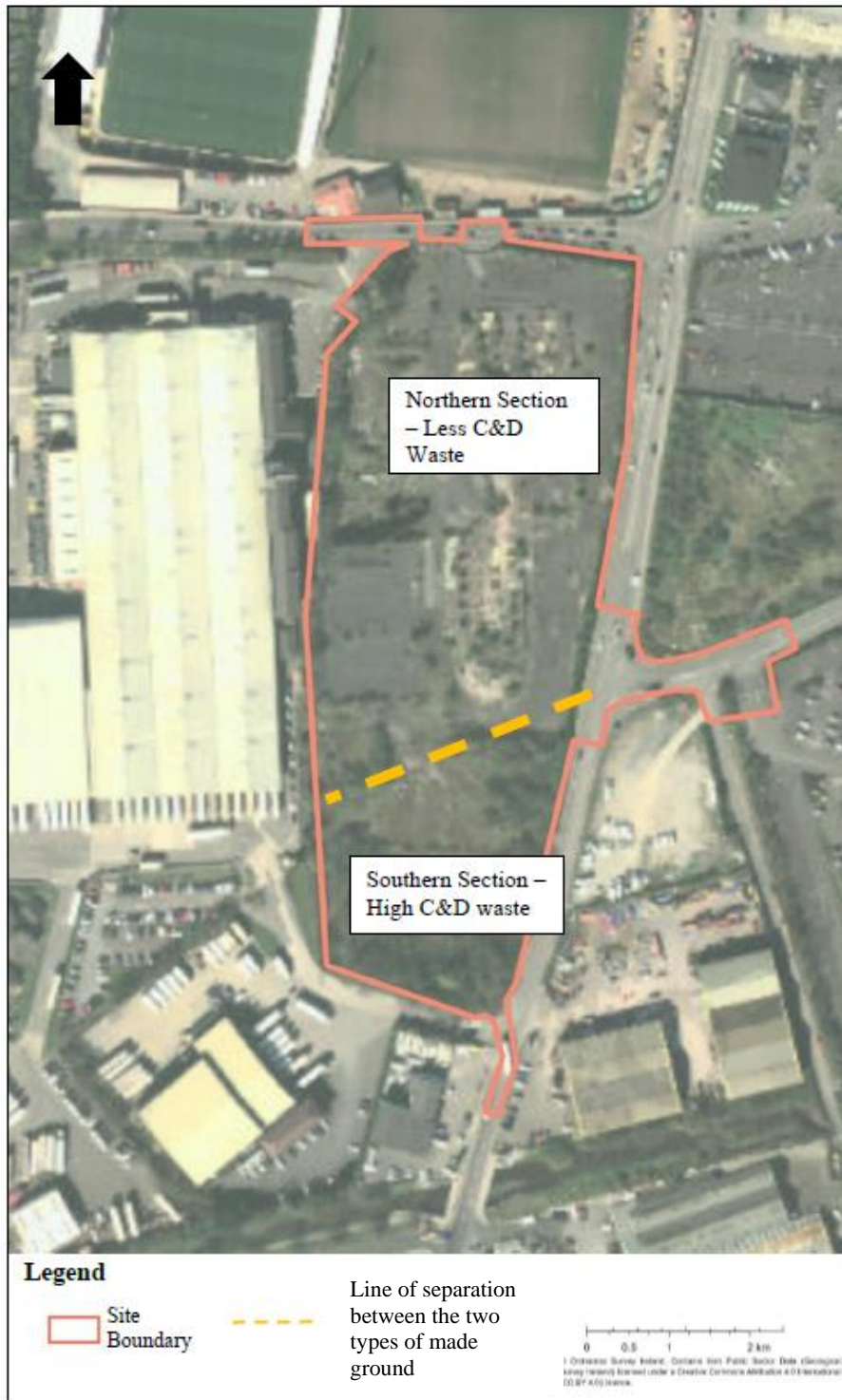
Figure 13.14 The line of separation between the made ground in the northern and southern sections of the site | not to scale
